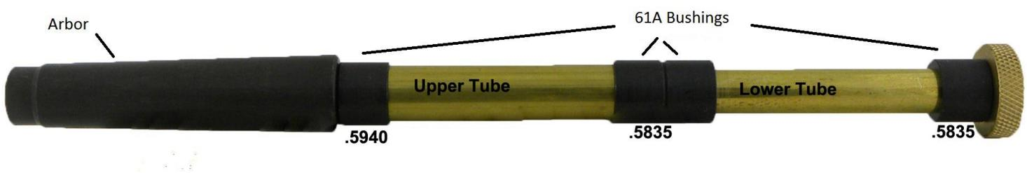
1. Assemble the blanks on the mandrel with 61A Bushings. The outside diameter on 3 bushings are the same size, the cap finial bushing is slightly larger than the rest.
